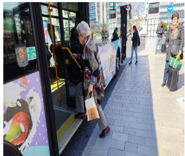
▲ Figure 5. Gap between the curb and the bus
