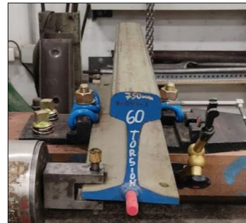
Rail fastenings: longitudinal & torsional resistance
