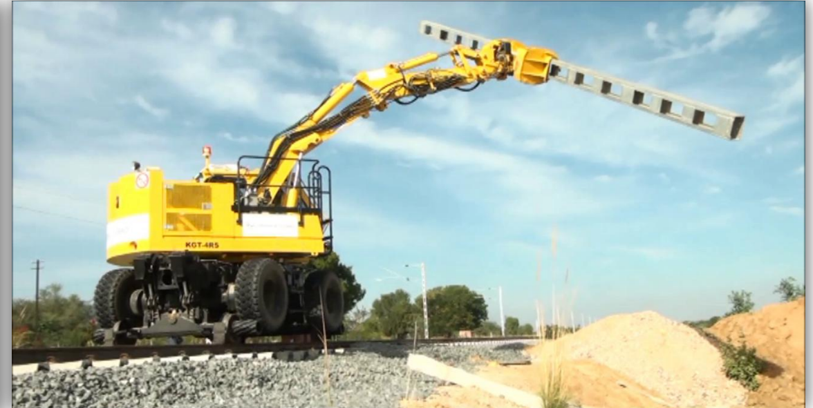
OHE Erection using Mast Grabber
