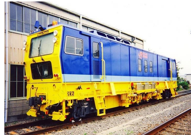
(4) Ballast stabilizing and measuring track irregularity
