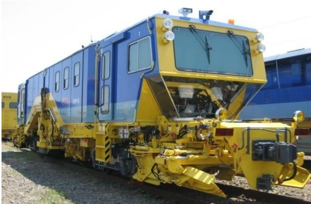
(3) Ballast distributing and profiling
