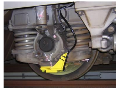
Longitudinal Irregularity and Axle Box Accelerometer
